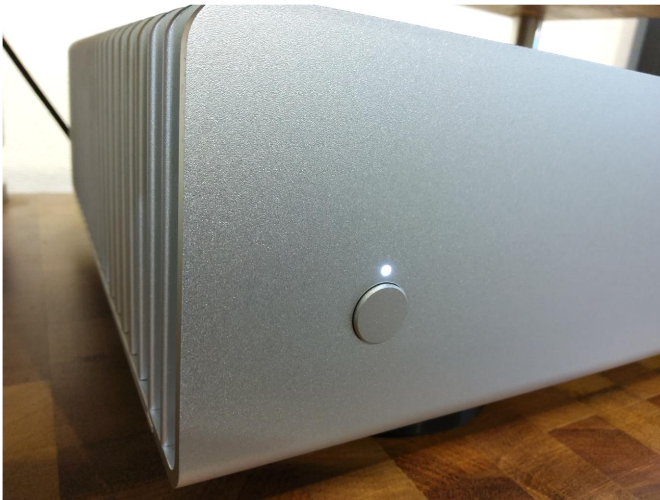
Figure 6 AARS soft power button and power indicator white LED
