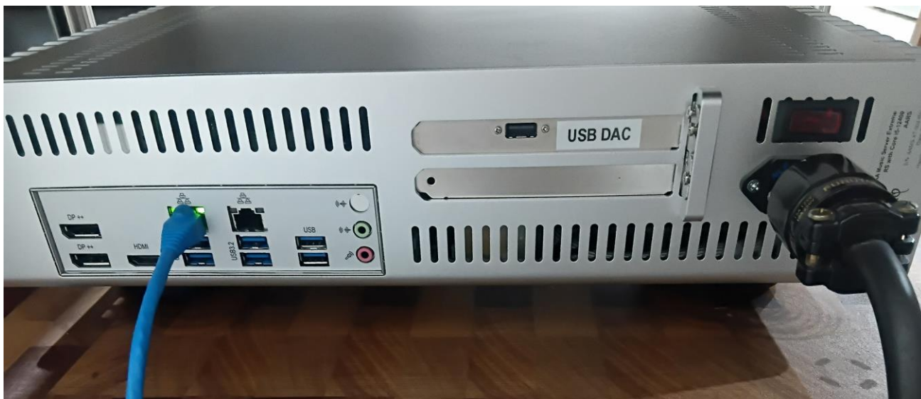
Figure 2 Wired LAN connection to the Motherboard
